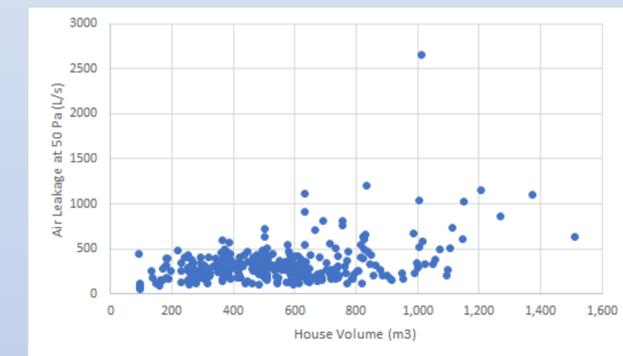
Figure 5: A plot of air leakage against house volume for prefabricated new homes.
