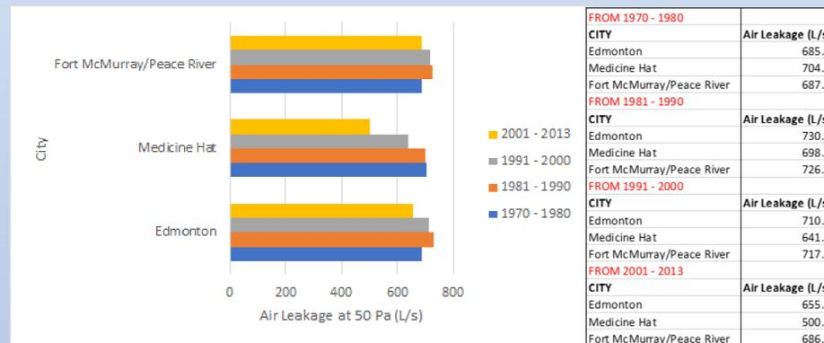
Figure 2: Closer look into 1970 to 2013 existing homes data. Air leakage versus City in Alberta.
