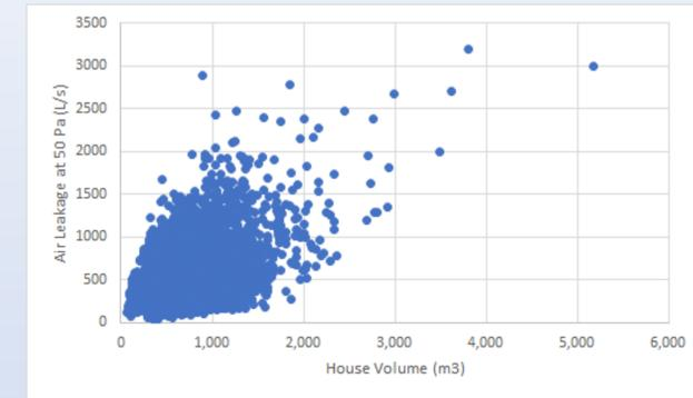
Figure 4: A plot of the air leakage against house size for stick built new homes.
