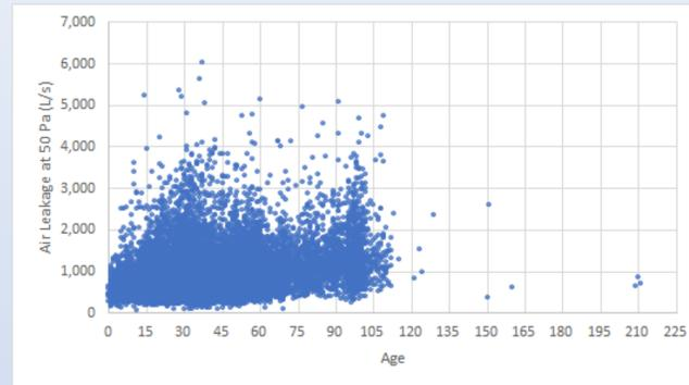
Figure 1: A Plot of air leakage (measured at a 50 Pascals pressure difference between indoors and outdoors in L/s) against the age of the existing houses. Data from houses located in Alberta.
