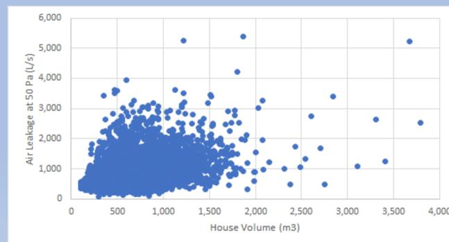
Figure 3: Graph of air leakage versus house volume for the years of 1980 to 2016. Data is from existing homes in Alberta.
