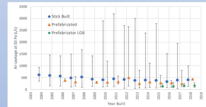
Figure 6: A comparison of air leakage for stick built, prefabricated homes. The ends of the error bars represent the maximum and minimum air leakage values in each of the years and the points are the average air leakage per year.
